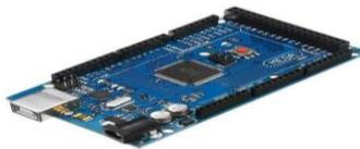
**Gambar 2. Arduino Mega**
